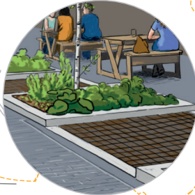
Baltic Close permeable paving and rain garden
